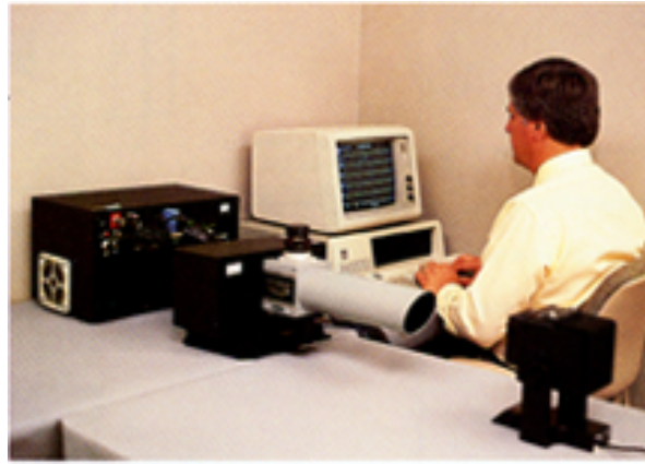
Aerospace Optics spectroradiometer used in measuring and certifying NVIS compatibility.
